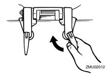
If the engine restraint cable attachment is equipped on your engine, an engine restraint cable or chain should be used. Attach one end to the engine restraint cable attachment and the other to a secure mounting point on the boat. Otherwise the engine could be completely lost if it accidentally falls off the transom.
